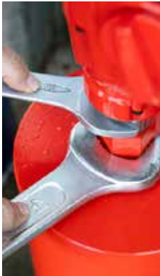
Mount Core Drill Ø 150 mm .... 3.7 kg
